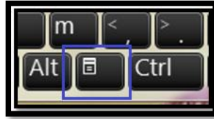
Figure 6 AppKey is located between the Alt and Ctrl keys on the right side of a QWERTY keyboard.
