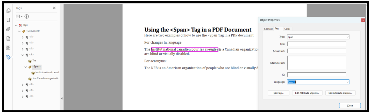
Figure 28 <Span> Tag used to identify the change in language for a sentence in PDF.
