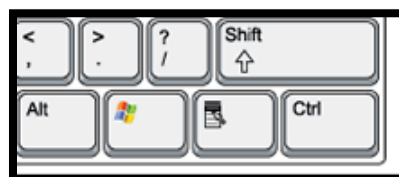
Figure 4 The AppKey is shown between the Windows and Ctrl keys on a standard keyboard.
